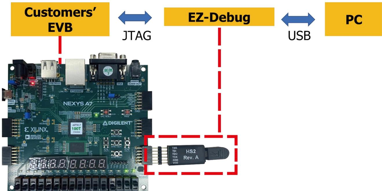
The figure below shows actual usage. The red box indicates the adapter cable, with the FPGA on the right side and the PC on the left side.
